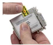
Remove the ink cartridge from packaging. Carefully pull the yellow tab tape from each cartridge
