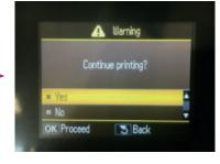
Using the buttons next to the LCD screen on the printer, move the up arrow to the YES position and press OK
