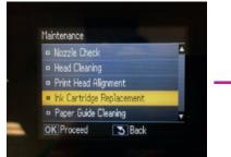
Using the arrows next to the LCD screen on the printer select > Setup > Maintenance > Ink Cartridge Replacement > Start
